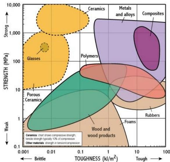
Figure 4 - Fracture Toughness of Materials
