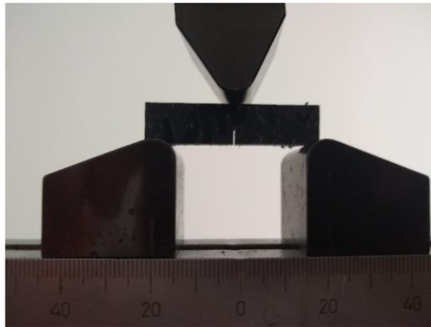
Figure 5 - Specimen used for fracture toughness testing
