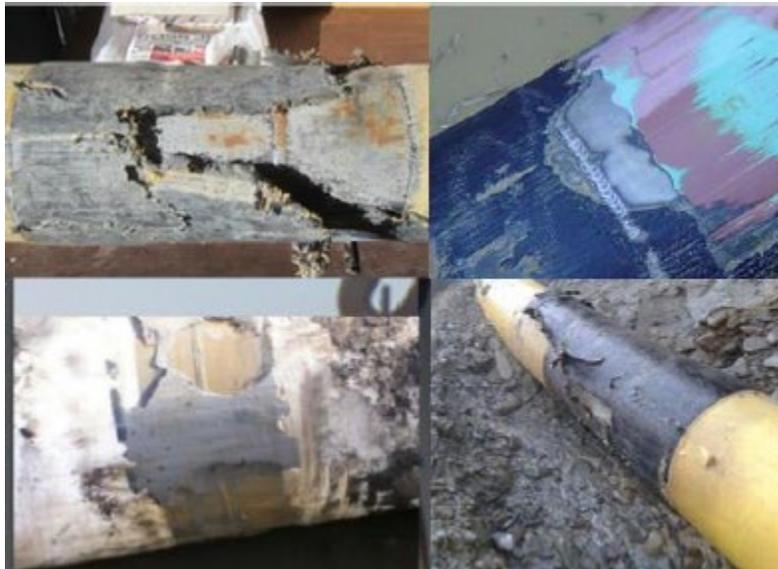
Figure 1 - Shearing, tearing, and opening failures
