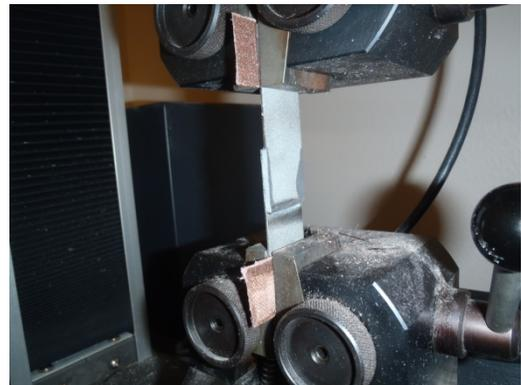
Figure 4: Testing of lap shear sample
