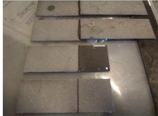
Figure 3: Lap shear sample preparation
