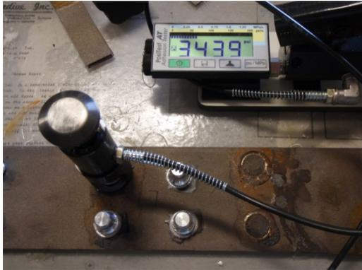
Figure 5: Dolly testing of bonded samples
