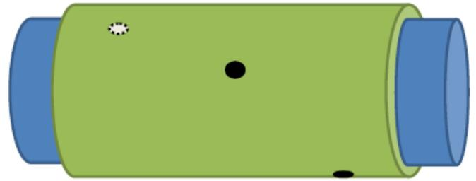
**Figure 2** - Orientation of 3 holiday test specimens (top left holiday on back side of sample)
