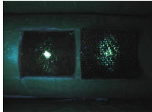
Figure 5 – Square of composite cut and under black light
