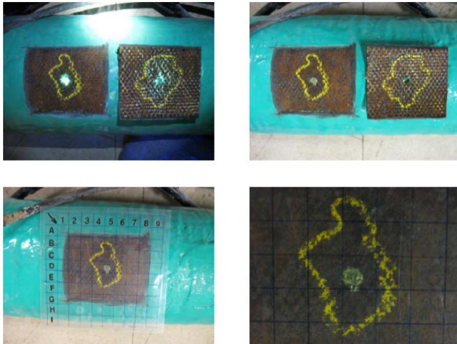
**Figure B.2** – Carbon/Fiberglass Sample 8: Disbonded area under black light (top left); Marking of disbonded area (top right); Disbonded area with grid layout (bottom left); Close-up of disbonded area with grid (bottom right)
