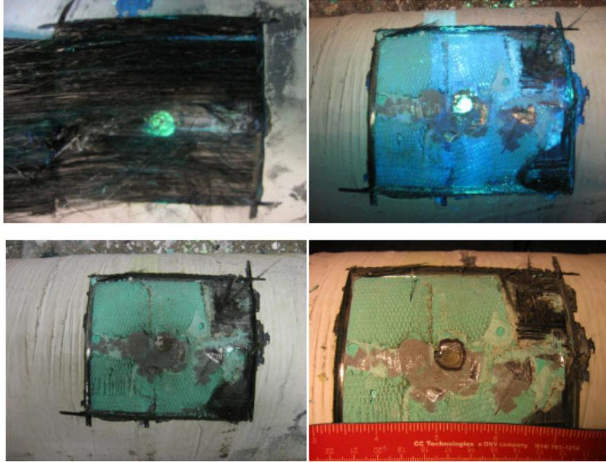
**Figure B.3** – Carbon Sample 9b: Removing composite square (top left); Disbonded area under black light (top right); Disbonded area (bottom left); Close-up of disbonded area with outline (bottom right)
