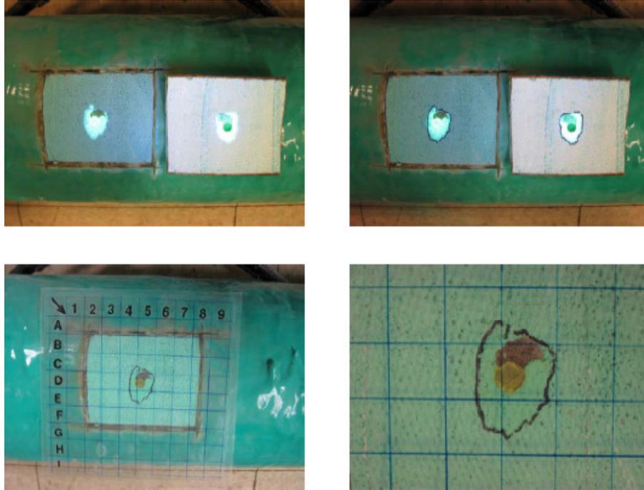
**Figure B.1** – Fiberglass Sample 2: Disbonded area under black light (top left); Marking of disbonded area (top right); Disbonded area with grid layout (bottom left); Close-up of disbonded area with grid (bottom right)
