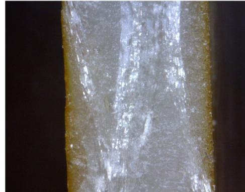
**Figure 4 - Cross Section of Tensile Coupon**
