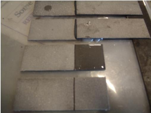
**Figure 2 - Creating the Lap Shear Test Pieces**
