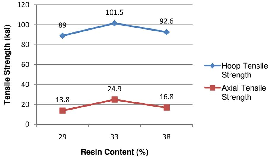
**Figure 9 – Tensile Strengths vs. Resin Content**
