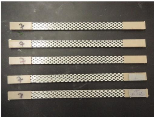
**Figure 3 – Tensile Specimens (before)**
