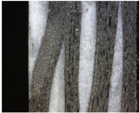
**Figure 2 – Edge of Sample Cut by Waterjet**
